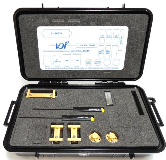
Figure 10: Type B TRL Calibration Kit Equipment typically supplied for Type A and Type B TRL calibration is shown at the left. This kit's label (above) is modified to reflect typical contents.
