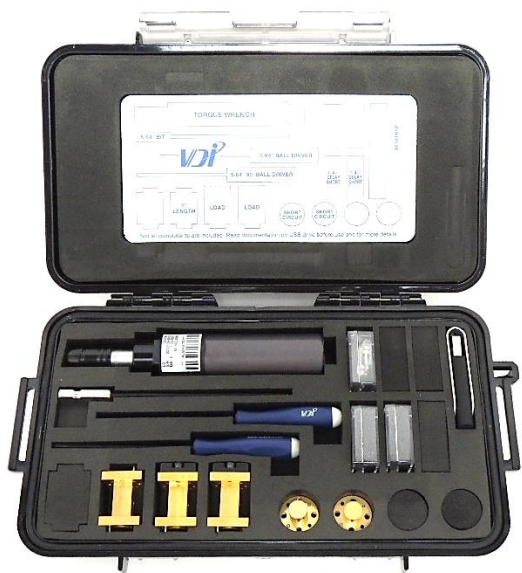
Figure 11: Type B SOLT Calibration Kit Equipment typically supplied for Type B SOLT calibration is shown at the left. This kit's label (above) is modified to reflect typical contents.
