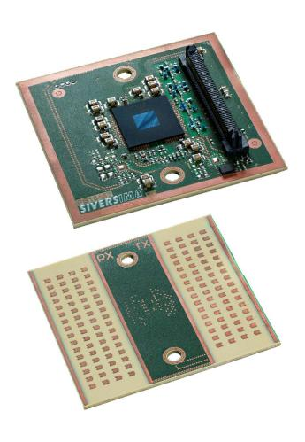
Why should you design the Radio Frequency part in your 60 GHz beamforming access product, when Sivers Semiconductors has done the work for you? Utilize the benefits of our RF modules BFM06010 and BFM06011. Unmatched power performance and throughput together with an integrated antenna gives you a competitive advantage in the unlicensed 5G race.
